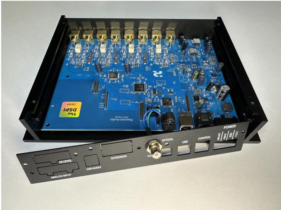
**Step 3.** The processor panel has windows for the connectors of external connections of newly installed modules, which are closed with plugs in the initial state. When installing the module, it is necessary to carefully, trying not to damage the board and processor elements, break out the corresponding plug to free this window.
