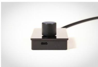
The Resolut SRC remote control can be installed both on the surface and by mortise mounting. For convenience, there are magnets on the back of the remote control, and a metal mounting plate is included. In the simplest case, you can fix the bar in any suitable place and fix the remote control on it with one movement.
