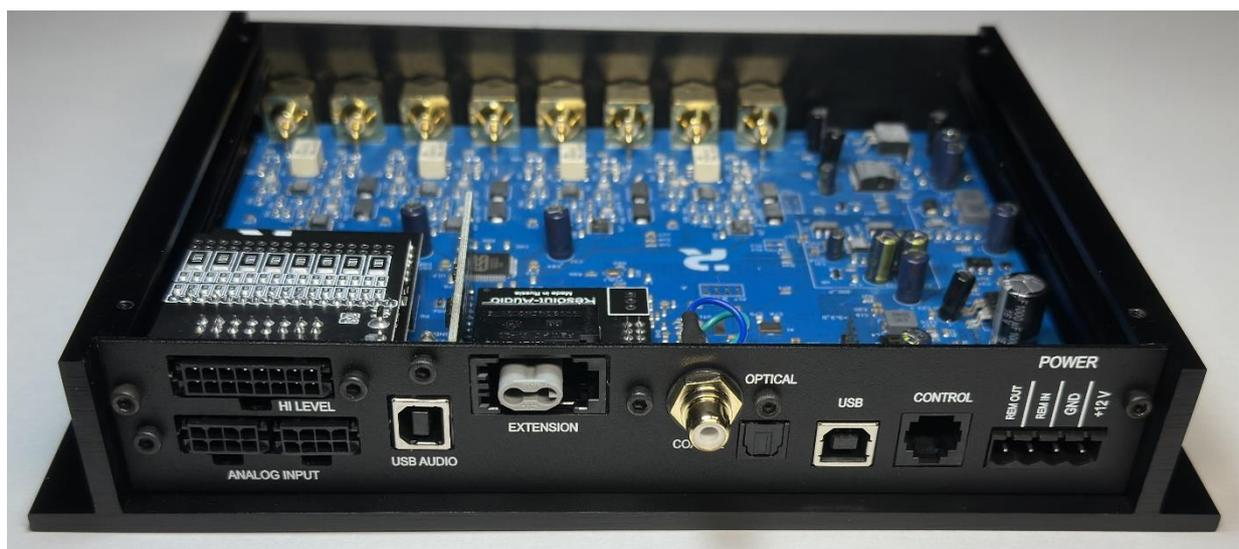
Make sure that the module is inserted tightly, all the contacts of the "comb" have completely entered their corresponding places on the module, and the connectors of the external connections of
